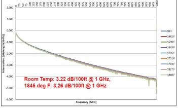
Attenuation - USA ROPE HEAT CLEANED 2" Pitch - UL2196 SMALL FURNACE Burn Lab Data
